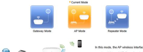
In this mode, the AP wireless interface and cable interface are bridging together. Without NAT, firewall and all network related functions.
