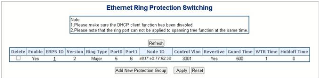
Figure 4-14-2: Ethernet Ring Protection Switching page screenshot
