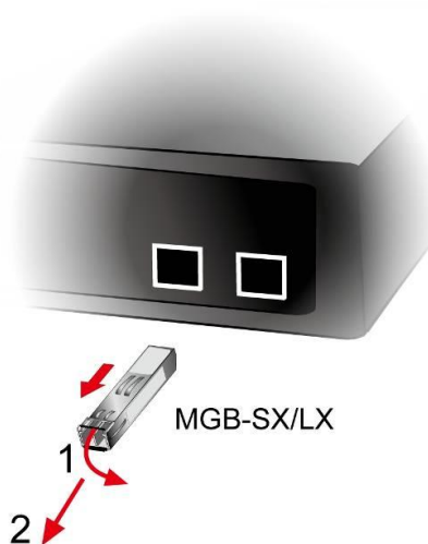
Figure 2-1-2g How to Pull Out the SFP Transceiver
