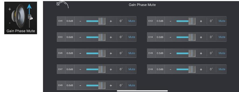
In this menu, you can make the following settings for each individual channel: volume, mute, and phase. Adjust the gain using the slider or the +/- buttons.
