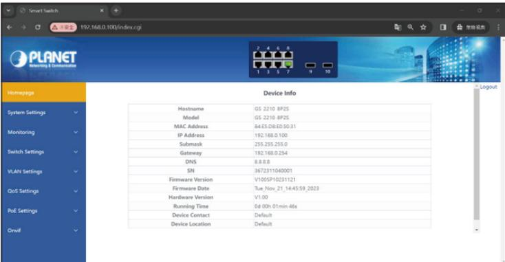
Figure 2-3: Web Main Screen of Web Smart Ethernet Switch
