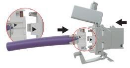
7. Insert wire manager into keystone body, ensuring that the arrow on both are aligned on the same side.
