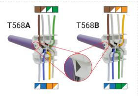
5. Insert wires through wire manager then secure each wire into its respective position.
