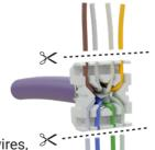
6. Cut off excess wires, taking care to cut flush to the wire manager.
