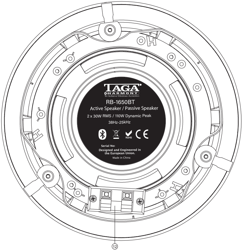
12. MASTER SPEAKER INPUT terminal - Spring Clips [+ and -]
