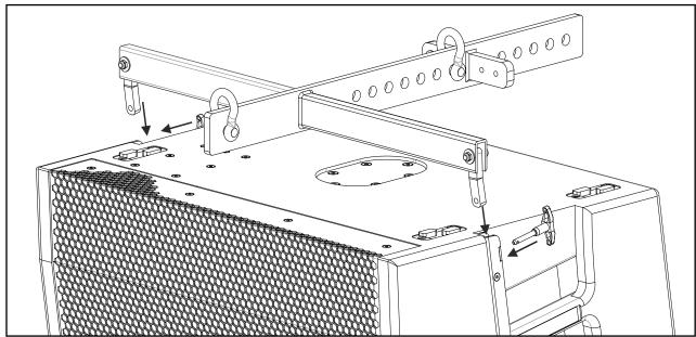
NOTE: Ensure all pins on all cabinets are inserted correctly and fully in their corresponding holes.
