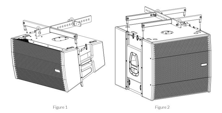
• When using the SV-CXA with the sub units (Figure 2) they are supported via 4 points with 2 lateral plates incorporated in each cabinet locked with two special steel pins per side.
