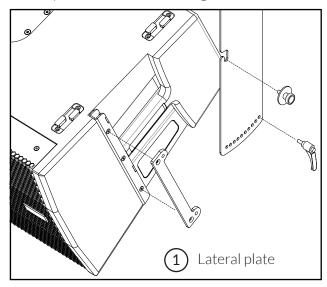
Just unscrew the upper and lower screws (don't touch the center screw) and retire these 2 screws from the cabinet. In their place you have to insert the screws DIN7991 5x50 (longer) provided with the UBR-CXA12 mounting kit.
