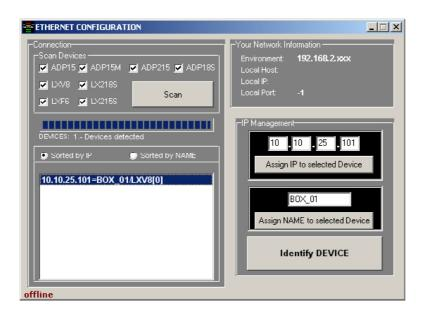
The Network environment consists in the first 3 sets of three numbers separated by dots. In order to detect/communicate with the cabinets, the software and the cabinets **must have the same Network settings**.
