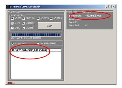
In this case, we can see that the cabinet do not have the same IP environment as the PC. So, select the cabinet and modify the assigned IP in order to be able to connect to it.
