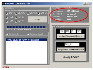
When we have a lot of cabinets connected in the network we can use the button "Identify Device" to see which box is selected (two activity LEDS will blink for one second). With that information then we can "Change NAME" assigned to this Cabinet by clicking in the "Assign NAME to select Device" button after writing in the box above the desired Name.
