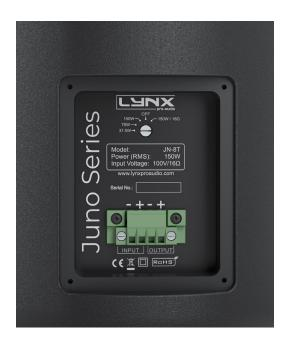
On the Juno-6T, the available power taps are 20W, 40W and 80W. On the Juno-8T, the available power taps are 37.5W, 75W and 150W.
