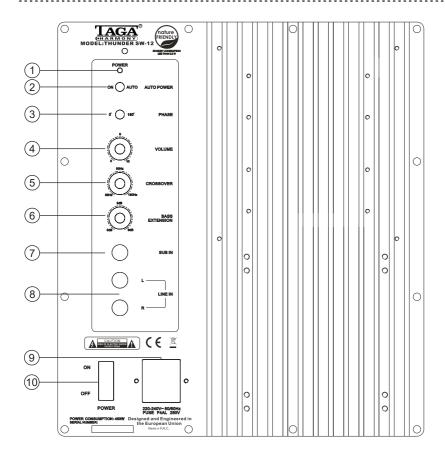
Available controls and inputs as well as their placement on the rear panel vary depending on the model. The above figure shows the Thunder SW-12 subwoofer rear panel.
