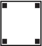
Placing the subwoofer in the corners usually gives much amount of bass but with less precision and definition.
