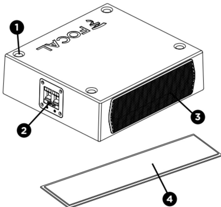
**1. Holes for attaching to the vehicle floor:** Please use suitable screws to avoid damaging the floor of your vehicle or any of its other components.
