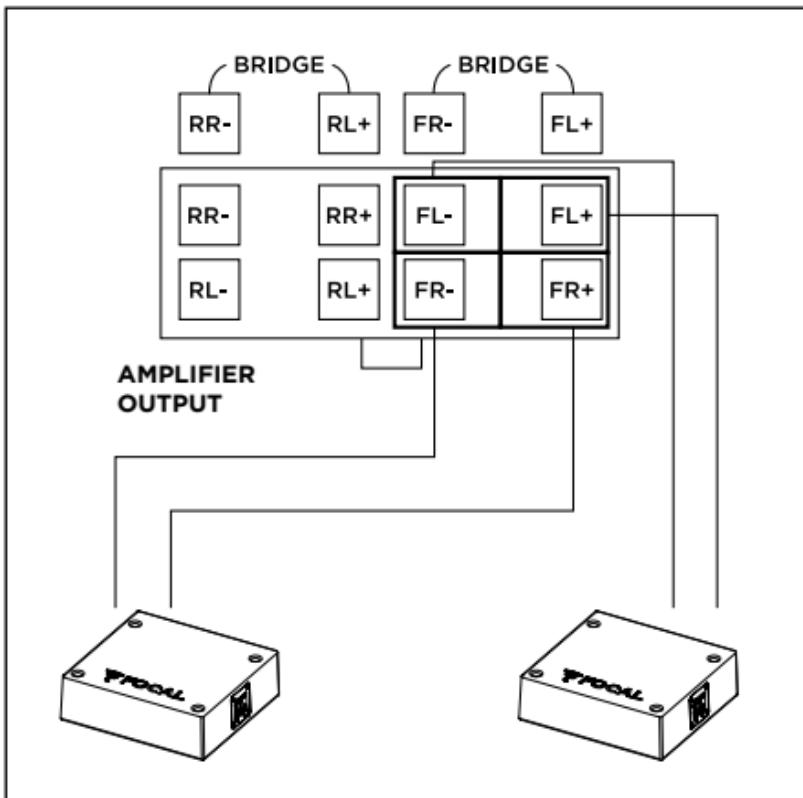
**WARNING:** Use an independent unbridged channel from your amplifier to supply each subwoofer. It is not advisable to use a parallel connection from both subwoofers or to connect them to a bridged output, as this could damage the amplifier.
