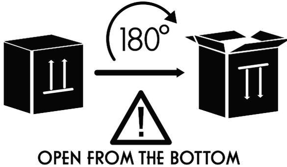
Place the carton with the subwoofer on the floor in the upside down position and open it from the bottom, remove the internal packaging which protects the subwoofer on the bottom. Carefully turn the carton with the subwoofer upside down. When the subwoofer is securely placed on the floor remove the carton and internal packaging - your subwoofer is ready for placement in your room.
