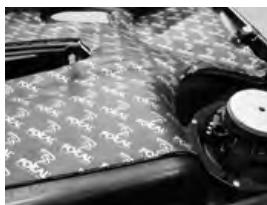
An acoustic insulation is needed to cancel the vibrations caused by the speaker fixing on the trim (ref. B.A.M.).
