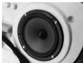
Focal speaker riveting (aluminum 4x16mm rivet).
