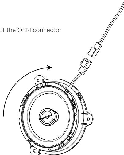
2 - Fix the speaker using the included rivets
