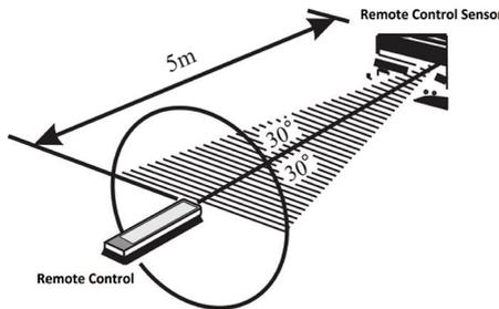
Use the remote control within a range of 5 meters from the amplifier and angles of up to 30 degrees aiming at the remote control sensor.
